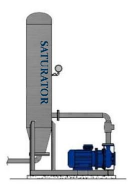
■ A recycle stream of treated effluent is taken from the discharge end of the GT-DAF and is pressurised to 450 kPa.
